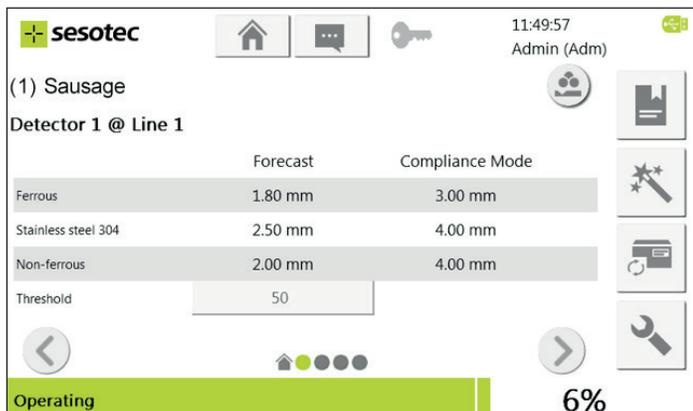
The screenshot shows the INTUITY CONTROL interface. At the top, it displays the 'sesotec' logo, a home icon, a message icon, a key icon, the time '11:49:57', and the user 'Admin (Adm)'. Below this, it indicates '(1) Sausage' and 'Detector 1 @ Line 1'. A table shows detection parameters for different materials:
